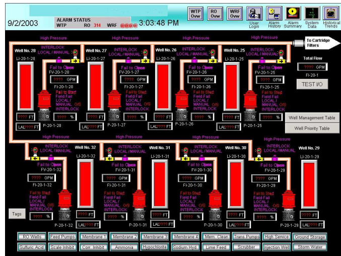
Figure 4 – An example of an RO Well HMI Screen
